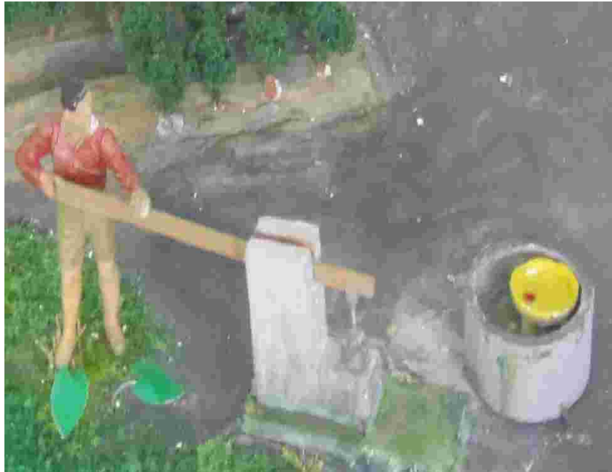
Hand pump and iron removal filter
