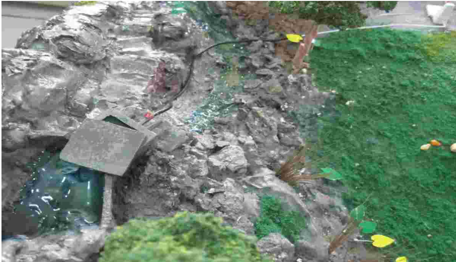
Spring box with transmission pipe, distribution pipe and tap stand.
